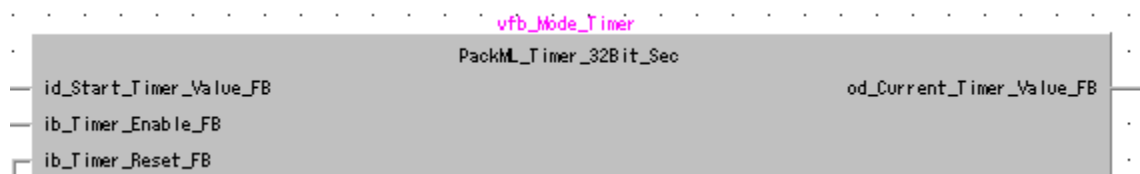
Figure 9 Timer_32Bit_Sec Function Block
