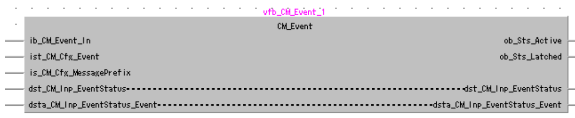
Figure 1 – CM_Event Function Block with Inputs and Outputs
