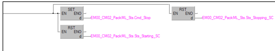
Figure 23 – Sample Ladder Logic for Handling PackML Commands
