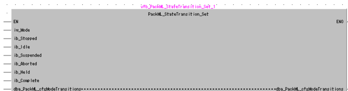
Figure 12 PackML_StateTransition_Set Function Block
